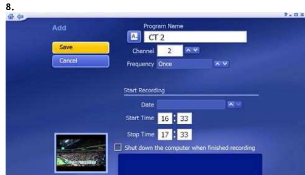
Adding to the list of scheduled records Select the program (program name), channel, date, start time and stop time. If you want to turn off the computer after recording, check box (shut down the computer when finished recording)
