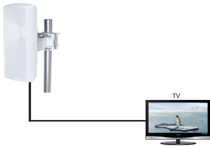
Installation 1: Directly connected to TV(Fig.6)
